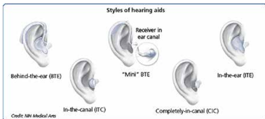
Figure 1. Styles of wearable hearing aids (from https://www.nidcd.nih.gov/health/age-related-hearing-loss )
